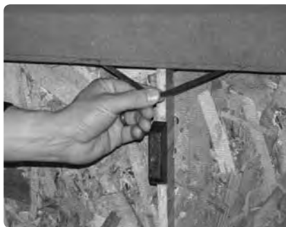
Reach up under the fabric edge, pull out the little elastic bands...
