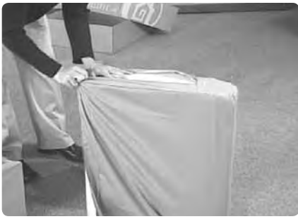
Working your way around the sides of the cushion pull the corners of the cover onto the foam...
