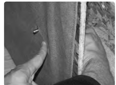
The arm is moved away from the frame in this photo so that you can see how the connector bolt protrudes through the circular hole cut in the fabric.
