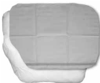
When filling the back cushion, match up the rounded corners of the back cushion with the rounded corners of the cover.
