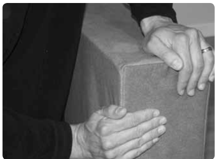
Once the arm cover is in place, smooth and straighten the fabric.
