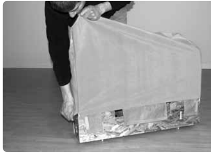
Now that you have the cover positioned onto the frame at both sides, you can begin to work the cover all the way down...
