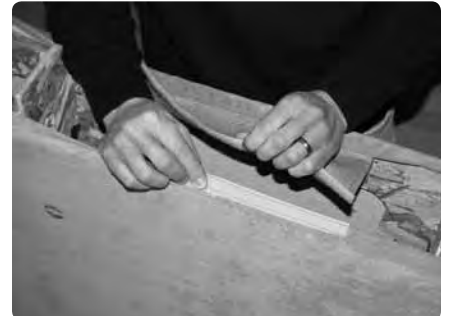
Starting with the flap in the middle, draw the sides of the arm taut by pulling up on the fabric, folding the flaps over...
