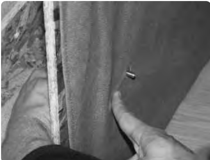
The arm is moved away from the frame in this photo so that you can see how the connector bolt protrudes through the circular hole cut in the fabric.
