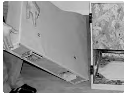
Now turn the arm over as well. Notice the holes in the arm fabric, they go up against the frame.
