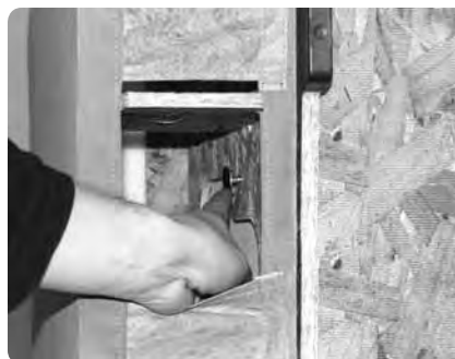
Now put the connector bolt that goes toward the front of the frame into place.
