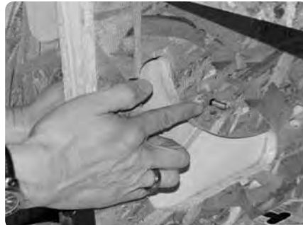
With the arm pushed against the frame, continue to insert the connector bolt through the frame as shown.
