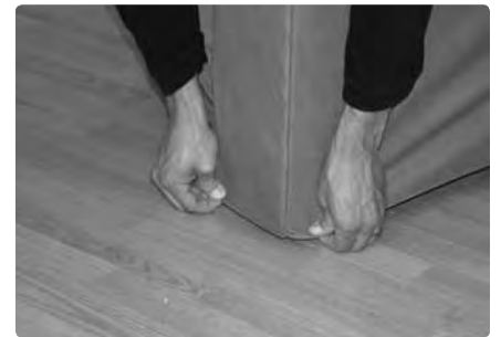
...aligning the cover seams with the edge of the frame and pulling each side alternately so that neither side gets too far ahead of the other.
