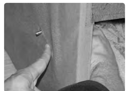
The arm is moved away from the frame in this photo so that you can see how the connector bolt protrudes through the circular hole cut in the fabric.
