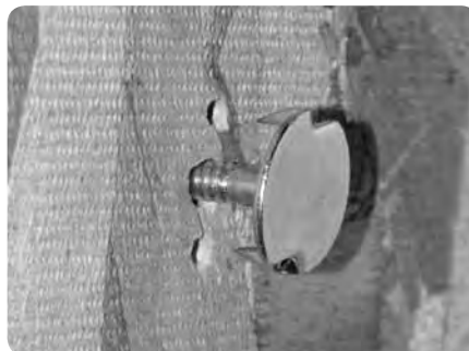
The two prongs on the connector bolt go into the two small holes. This keeps the bolt from turning.
