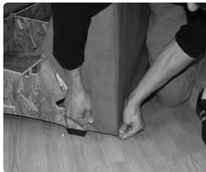
Wrap the cover around and under the back corner of the frame.
