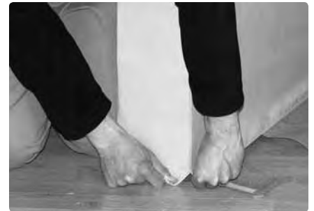
... aligning the cover seams with the edge of the frame and alternately pulling each side so that neither one gets too far ahead of the other.
