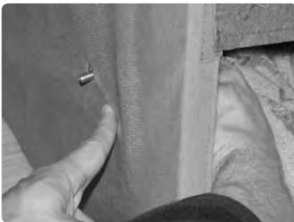
The arm is moved away from the frame in this photo to show how the connector bolt protrudes through the circular hole cut in the fabric.
