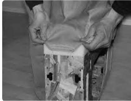
... and place it over the foam and frame.
