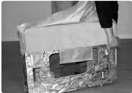
Then, position the cover and seams over the other end of the arm frame and work it down slightly...
