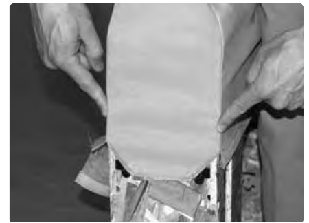
Align the seams with the edges of the wood arm frame and pull the cover down an inch or two onto the frame...
