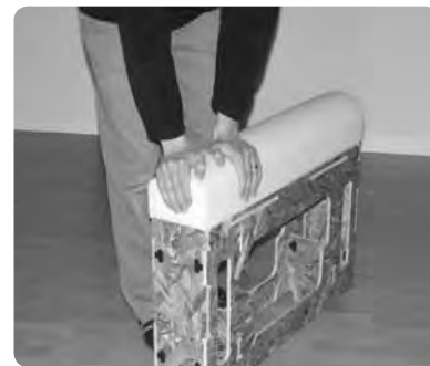
The bottom of the foam is recessed in order to fit onto the arm frame.
