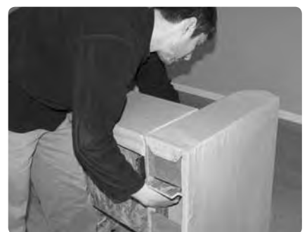
Once the connector bolts are in position at both front and back, tighten the wingnuts to draw the frames together.
