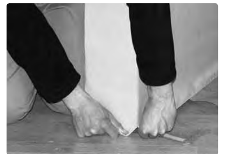
... aligning the cover seams with the edges of the frame and alternately pulling each side so that neither one gets too far ahead of the other.
