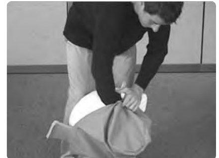
Then, turn the arm over and smash the foam down so that you can slip the foam inside the other end of the cover. It helps to stand in order to use your weight to smash the foam down.
