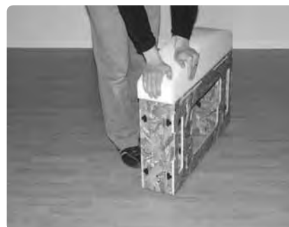
The bottom of the foam is recessed in order to fit onto the arm frame.
