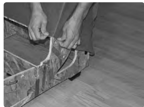
Pull the cover down, aligning the cover seams with the edge of the frame.
