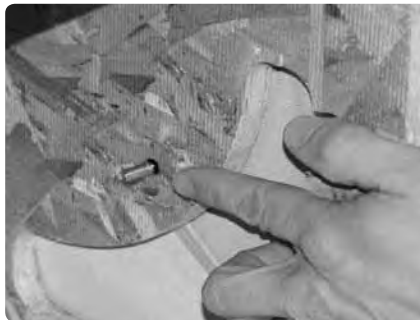
With the arm pushed against the frame, continue to insert the connector bolt through the frame as shown.
