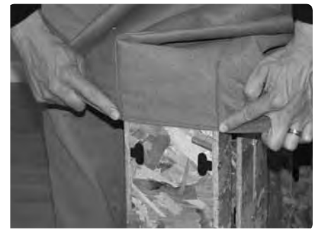
Align the seams with the edges of the wood arm frame and pull the cover down an inch or two onto the frame...
