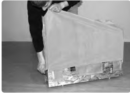
Now that you have the cover positioned onto the frame at both sides, you can begin to work the cover all the way down...
