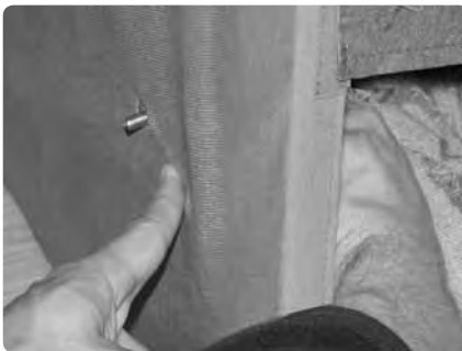
The arm is moved away from the frame in this photo to show how the connector bolt protrudes through the circular hole cut in the fabric.
