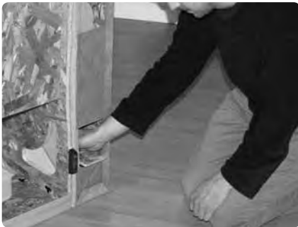
Follow the next steps to attach the connector bolt at the back of the frame (the hole closest to the floor with the frame on its back).
