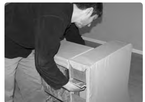
Once the connector bolts are in position at both front and back, tighten the wingnuts to draw the frames together.
