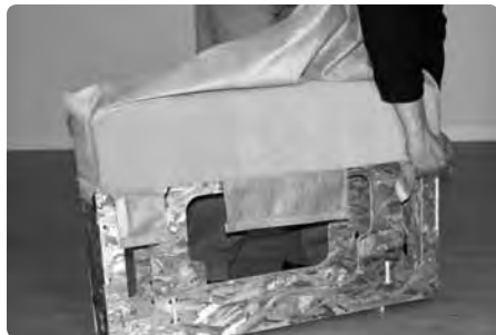
Then position the cover and seams over the other end of the arm frame and work it down slightly...
