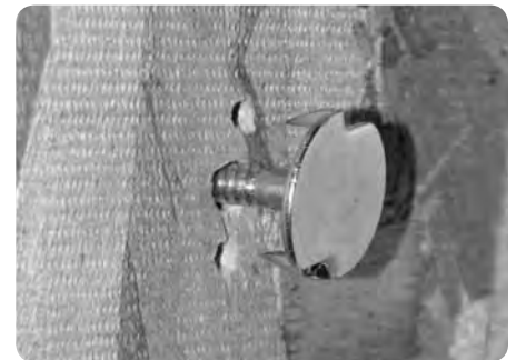
The two prongs on the connector bolt go into the two small holes. This keeps the bolt from turning.
