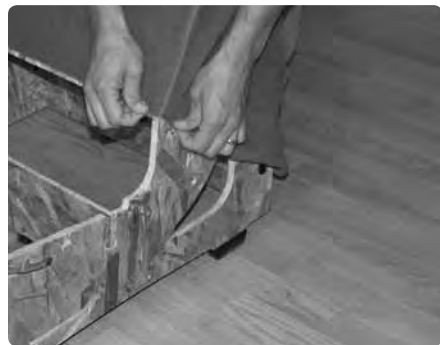
Pull the cover down, aligning the cover seams with the edge of the frame.
