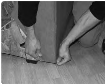
Wrap the cover around and under the back corner of the frame.
