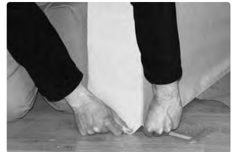
... aligning the cover seams with the edges of the frame and alternately pulling each side so that neither one gets too far ahead of the other.
