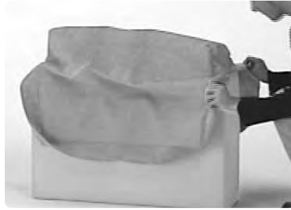
Position the cover over the foam and align the corners of the foam cushion with the corner seams of the cushion cover.
