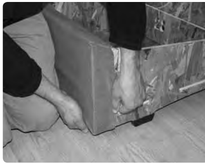
... and then pull the bottom corners of the cover around the bottom of the wood frame.
